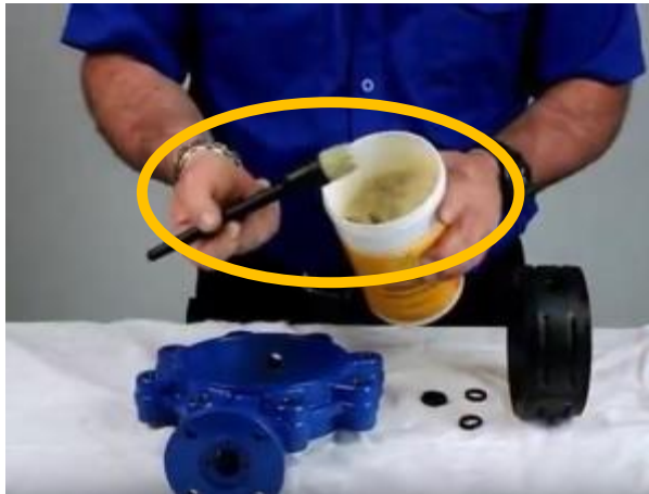
Maintenance of a valve flap
